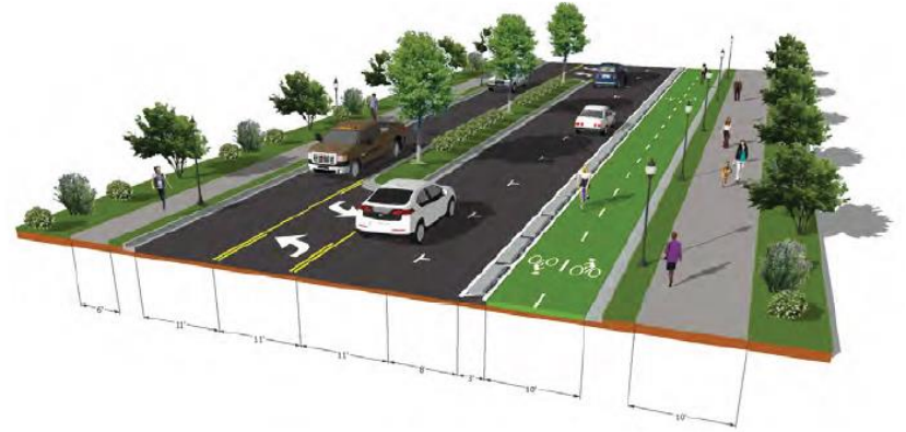
FIGURE 7.2: PROPOSED CROSS SECTION - MARSHALL WAY
